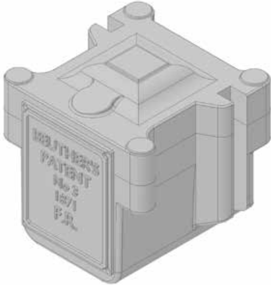
CAD view of the Axle box pattern to be made. Sam Palmer
