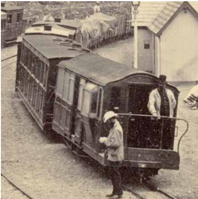
iBase image 3203 showing the buffer arrangement on Curly Roof Vans in the 1870’s. FR Archives
