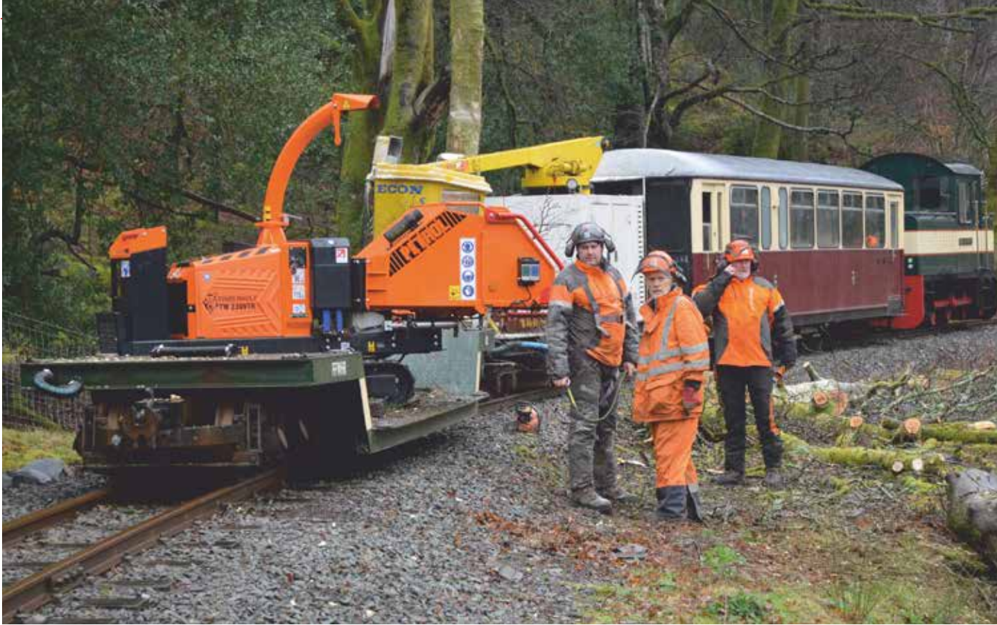
A wonderful illustration of the Well Waggon in use with the chipper loaded and the team posing on the Deviation. Here it is paired with Criccieth Castle and retired observation carr 111 as a mess van, one that is in need of modernization. David Firth
