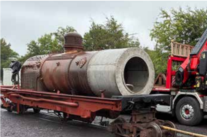
138’s boiler, now returned from rebuild and mated with its frames
