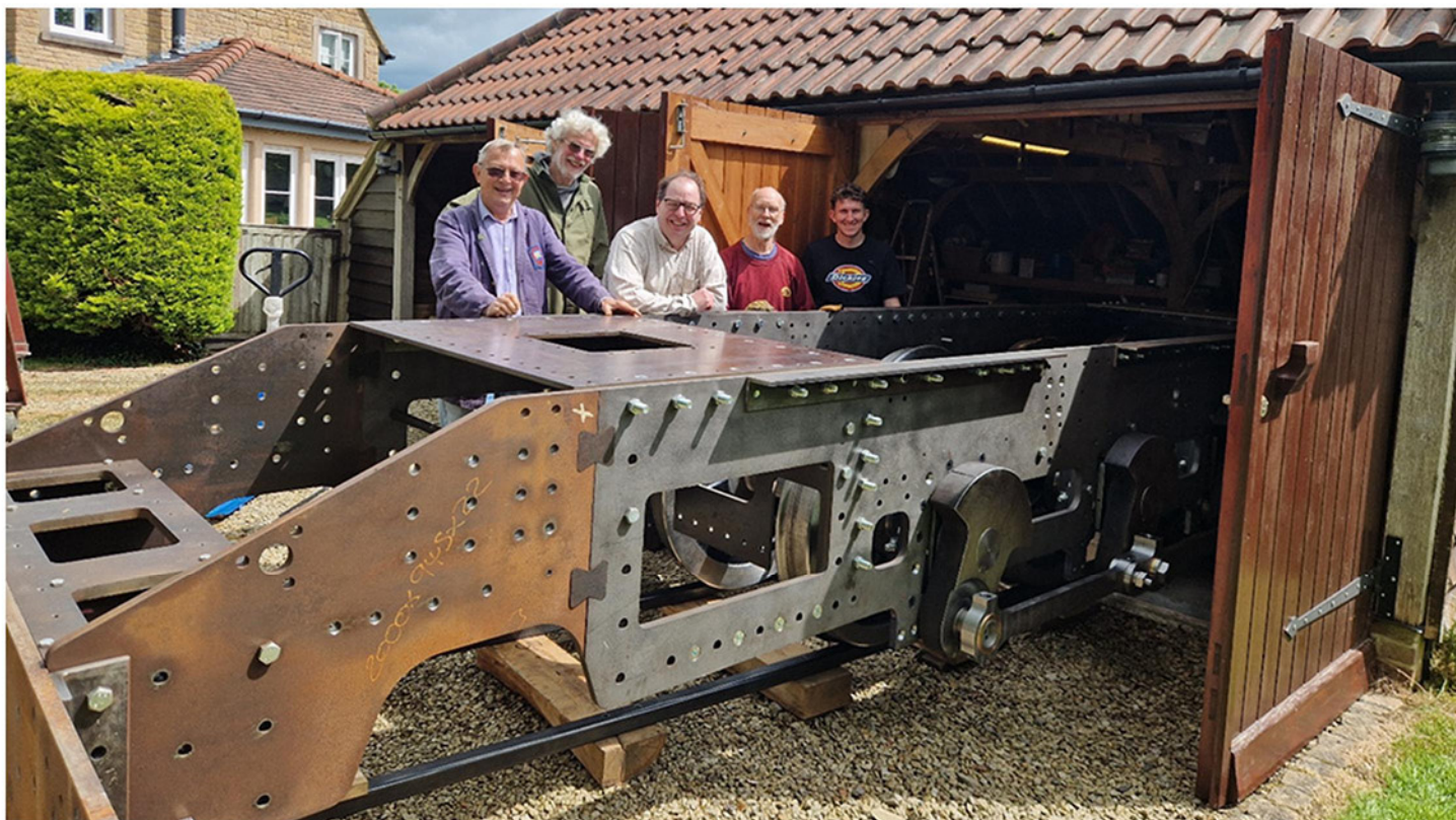
The frames rolled outside Jon's shed, with the main team behind the project build - consisting of Stuart, Roger, Jon, Alan and Josh. The frames have been made in three sections - partially due to the shed's size, but also due to cutting machine constraints.
