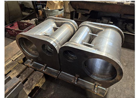
Driving wheels, rear pony truck & cylinder fabrications for the ZA/6. Middle: Matt Fairweather's 7¼" gauge Balson Furka HG 3/4. This is a compound loco, featuring Walschaerts (Heusinger) valve gear on the adhesion engine and Joy gear for the pinion engine.
