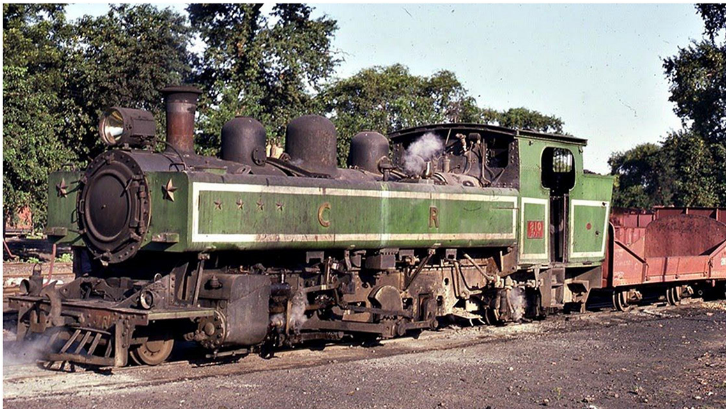
Photo of one of the ZA/5 Dholpur locos in India. Notable are the stars on the front and side of the water tanks which were awarded for reliability. The cabside plate displays the running number - 810 - and the type - ZA/5
