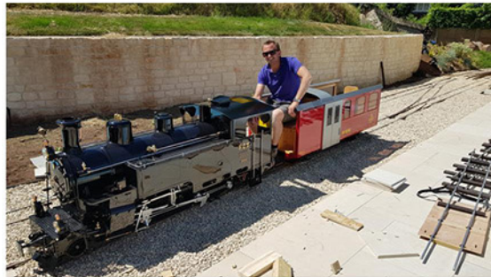
Driving wheels, rear pony truck & cylinder fabrications for the ZA/6. Middle: Matt Fairweather's 7¼" gauge Balson Furka HG 3/4. This is a compound loco, featuring Walschaerts (Heusinger) valve gear on the adhesion engine and Joy gear for the pinion engine.
