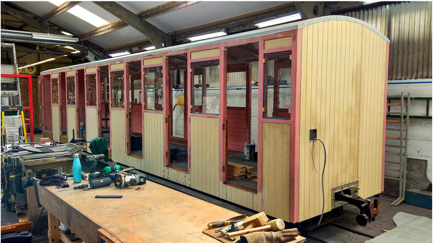
Carriage No.26 inside Boston Lodge Carriage Works on 12th August 2025 - note the adaptation being made to the furthest end of the carriage to provide an accessible doorway for wheelchair users. Roger Dimmick
