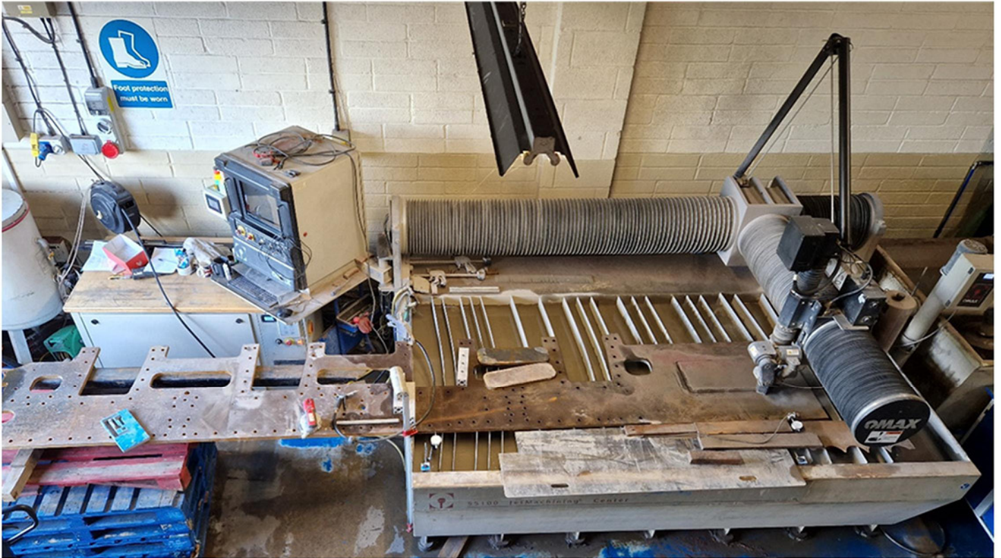
This picture shows one side of the main frame sections on the high pressure water-jet cutting machine. It is hard to over-emphasise how accurate these are - especially given the need to turn the steel plate halfway through the operation and maintain alignment.
