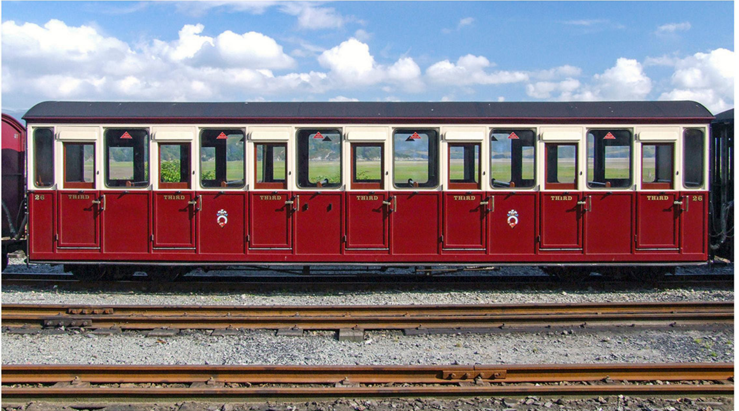
Carriage No.26 in Harbour Station sidings on 27th July 2006 - looking in good condition following a repaint during winter 2005, and giving a clear view of the redesigned body that had been fitted to the original underframe in 1986. Roger Dimmick
