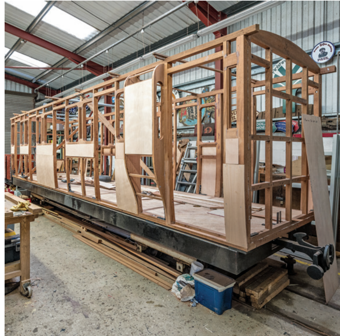
A replica of an 1870s Ashbury brake-composite carriage is being built for the Welsh Highland Railway's heritage fleet by Boston Lodge Carriage Works. (John Dobson)
