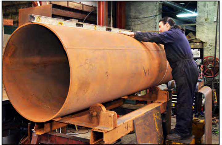
Top: The boiler barrel is prepared for assembly
